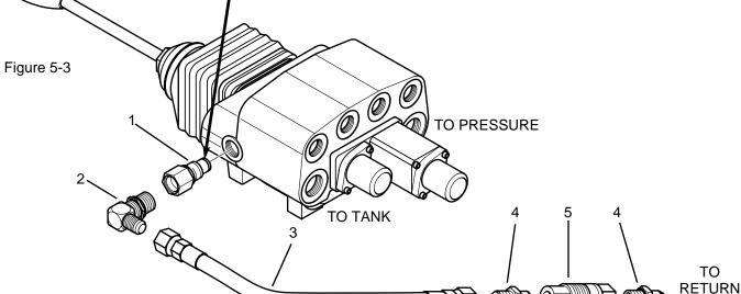
IMPORTANT: When Loader hydraulics are disconnected from tractor, the tractor hydraulic circuit must be completed by connecting pressure port to return port. Failure to do this will cause serious damage to tractor hydraulic pump.
